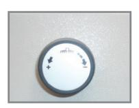
▲ Electronic hand wheel for backgauge position with variable speed (from very slow to very fast)
